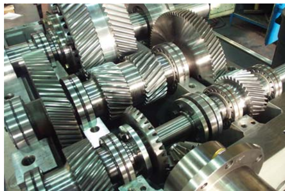
Through hardened precision manufactured helical gearing provides exceptional wear-in properties and a high resistance to unexpected shock loads.
