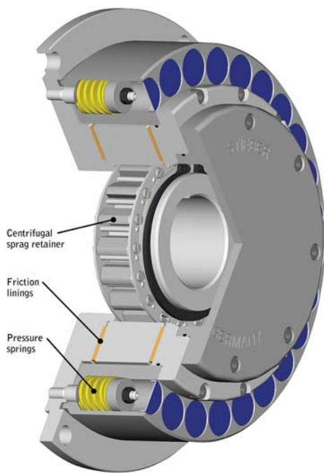
High-speed backstops are mounted on the high/medium speed shaft of gear drives on inclined conveyors or rotary machines such as crushers or kilns. When the drive is running, the input/output components of the backstop work contact-free and therefore contribute to a reduction in power loss.
