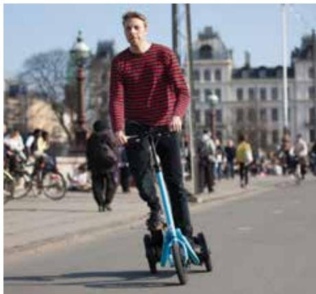
The Me-Mover step-driven transport vehicle provides users with a fun, active and energizing way to get to their destination. Riders use stepping motion, an oscillating movement of the pedal (up/down), instead of a rotating movement.
