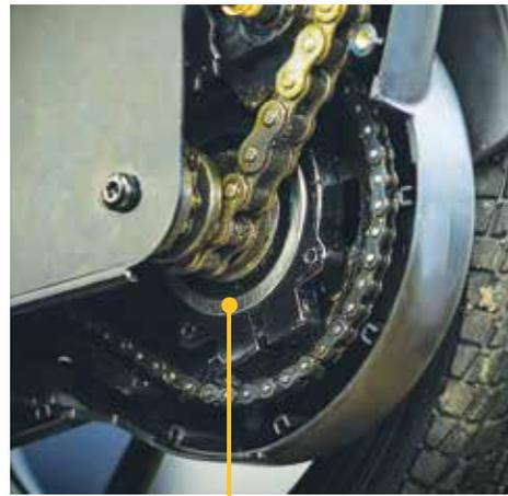
The drive wheel rotates in one direction only, so a freewheel (clutch) is needed to connect the transmission and the drive wheel – just as on a bicycle.
