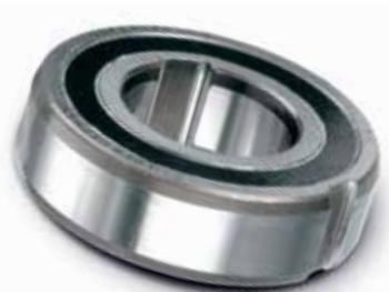
The Stieber Model CSK30 PP overrunning clutch features ultra-hard Formchrome® sprags which provide extra-long life, maximum wear resistance and lower maintenance costs. Formchrome sprags – exclusive to Stieber/Formsprag – are made by diffusing chromium into the surface of hardened high carbon alloy steel to form a chromium-carbide alloy.
