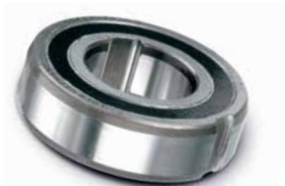
The Stieber Model CSK30 PP overrunning clutch features ultra-hard Formchrome® sprags which provide extra-long life, maximum wear resistance and lower maintenance costs. Formchrome sprags – exclusive to Stieber/Formsprag – are made by diffusing chromium into the surface of hardened high carbon alloy steel to form a chromium-carbide alloy.
