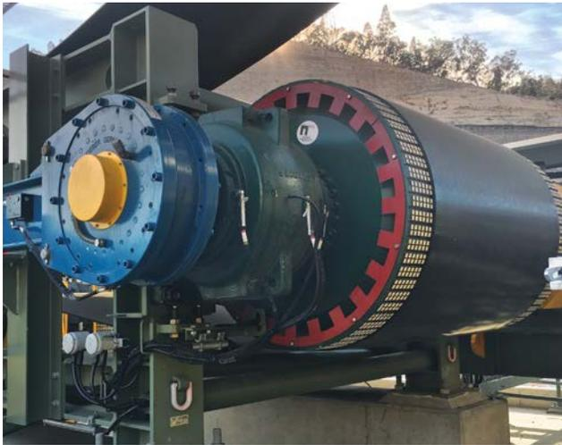
Dual RDBR 300 models with 70 kNm torque per unit are installed on the 1800 mm (5.9 ft.) wide, 3,050 m (1.9 mile) long drift conveyor at the Moolarben mine that transports coal from the longwall system underground to the surface. The inclined conveyor features an 80 m (262 ft.) lift and has a capacity of 4,500 tph.
