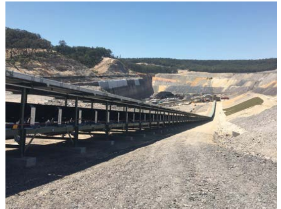
Twin RDBR 360 models with 120 kNm torque per unit are utilized on the ramp conveyor at the Moolarben coal mine. Advanced release functionality allows for controlled release of the tension on a jammed belt with unlimited backward rotations.
