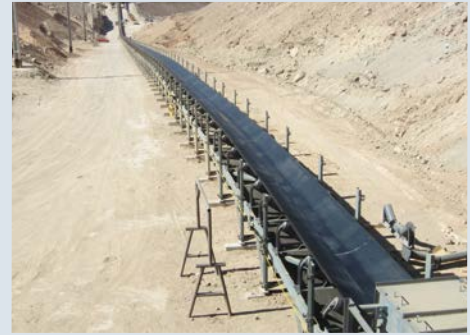
A large copper mine in Chile utilizes a series of three downhill in-line conveyors. Two of the conveyors are 1600 m (1 mile) long and the third is 700 m (.4 mile) long. The conveyors can transport 5,000 tonnes/hour with a belt speed of 5.5 m/s (12.3 mph).
