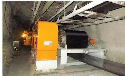
The brake disc diameter needed to be relatively small since space was very limited in the underground installation area.
