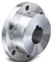
Amerigear FS207 hubs supplied have an 86,083 ft.lb. torque capacity. The units consist of a rigid (keyed) half that is mounted to the brake disc. The couplings were modified to accommodate a longer rigid hub engagement (length).
