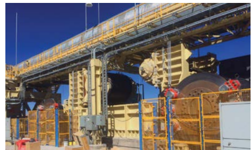
The entire four-flight, direct drive OGP1 conveyor system spans 10,632 m (6.6 miles) in length with the largest section being 3,942 m (2.4 miles) long.
