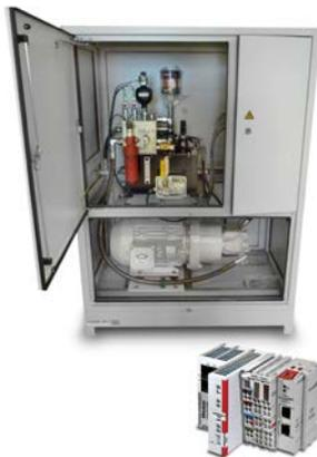
Pairs of SOBO® controllers and SOBO® hydraulic power units were installed on the OLAP conveyors. All Svendborg Brake power units are designed and manufactured in-house to ensure compatibility with other Svendborg braking system components. Units are equipped to monitor oil level and temperature, motor and pump function, and system pressure.
