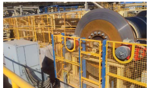
Pairs of Model BSFB 650 spring-applied, hydraulically-released, dual-spring caliper brakes, acting on 2.7 m (8.8 ft.) diameter steel brake discs, are positioned at the tail of the various OGP1 conveyor flights.
