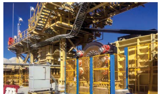
Groupings of six Model BSFB 650 spring-applied, hydraulically-released, dual-spring caliper brakes, acting on 2.7 m (8.8 ft.) diameter steel brake discs, serve as on/off holding brakes at the head of the various OGP1 conveyor sections.
