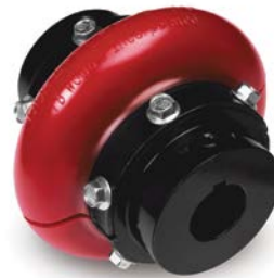
TB Wood's Dura-Flex couplings employ a light-weight element that absorbs shock loading and torsional vibration. A specially formulated elastomeric material offers superior chemical, dynamic, and weathering properties.
