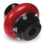
TB Wood's Dura-Flex couplings employ a light-weight element that absorbs shock loading and torsional vibration. A specially formulated elastomeric material offers superior chemical, dynamic, and weathering properties.
