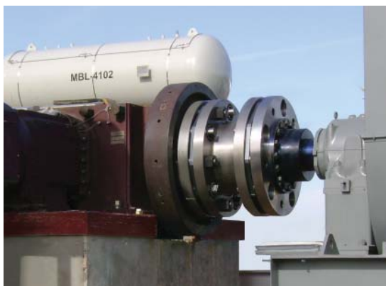
The largest coupling ever designed by TB Wood's transmits 10,000 HP to drive compressors that safely pump natural gas into and out of Louisiana salt dome facilities operated by PetroLogistics, LLC.
