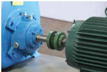
TB Wood's Sure-Flex® Plus non-spacer coupling, size 6, installed on Summit/GPM self-priming pump unit. This low rpm/high torque motor would normally require a size 7 coupling.
