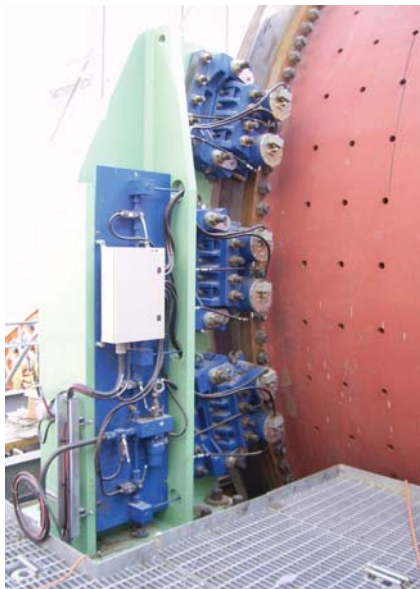
Each of the 8m ball mills utilizes six of the VMSDP brakes, providing a total braking force of 4.4 MN or 737 KN per brake.
