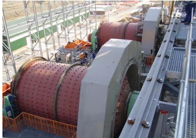
Two 8m diameter by 11.7m long gearless ball mills, both rated at 17.5 MW are among the largest in the world.
