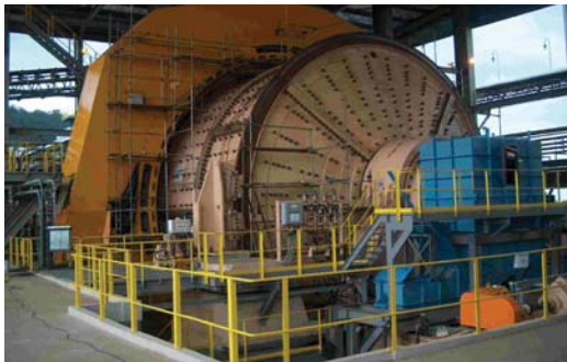
Figure 1: Sossiego 38' x 23' Long SAG Mill
