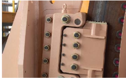
Figure 8: VMS-DP Caliper Assembly (showing reactive backplate)
