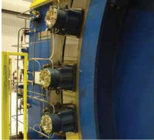
Twiflex Ltd. supplied eight VMS-DP brake calipers (with pedestals) plus a hydraulic power pack for each of the two primary mills.
