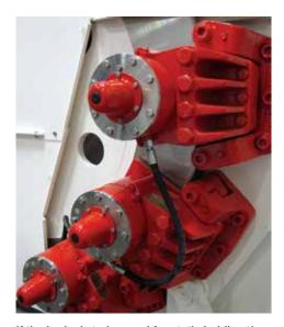
If the brake is to be used for static holding then bedding-in may not be possible so engineers should allow for reduced friction potential in the original design.
