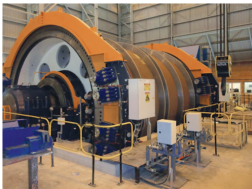
Twiflex provided parking brakes for use on mine hoists at the Nkana site of Mopani Copper Mines in Zambia.
