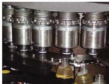
One bottling line at a Pepsi plant in Detroit uses 20 Warner Electric headsets to put caps on, letting the line crank out 1,000 bottles/min. A smaller line with 16 headsets handles 700 bottles/min.
