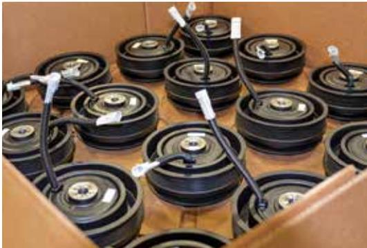
A variety of electromagnetic clutches and brakes, including PTO clutches and brakes for use on consumer and commercial lawn tractors, agriculture equipment and diesel engines are manufactured at the new plant.
