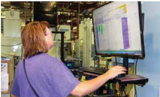
Associates now enter cell performance data details directly into an electronic visual management system for automated summation of near “real time” performance data. Large monitors, positioned next to the cells, display color-coded data for easier viewing by team leaders and supervisors.
