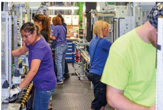
Work cells throughout the plant are ergonomically designed and arranged with CNC machines and part trays positioned for convenient access by operators.
