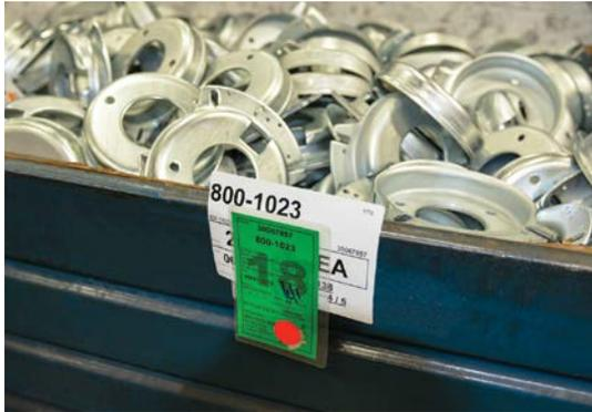
Kanban cards, attached to all material containers, indicate quantities, descriptions, etc. allowing anyone to easily access correct materials.
