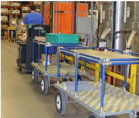
All raw materials and finished goods at the plant are delivered and retrieved utilizing a unique trolley train system that cycles through the plant every two hours.
