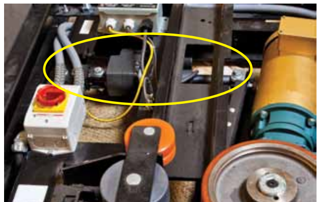
When activated, the Warner Linear actuator pivots the motor drive carriage into position under the carousel center chain, allowing the friction wheels to engage and drive the chain. When the controller shuts down a motor, the actuator disengages the friction wheels of the motor away from the center chain, so that the de-energized motor doesn’t become a source of drag.
