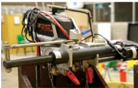
Warner Linear actuators are used to turn the two outboard motors on the unmanned vessel.
