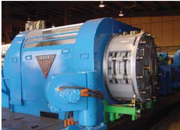
Tri-Service Oilfield Manufacturing (TSM) incorporates the Wichita Clutch Dual-Actuator AquaMaKks on their drawworks.
