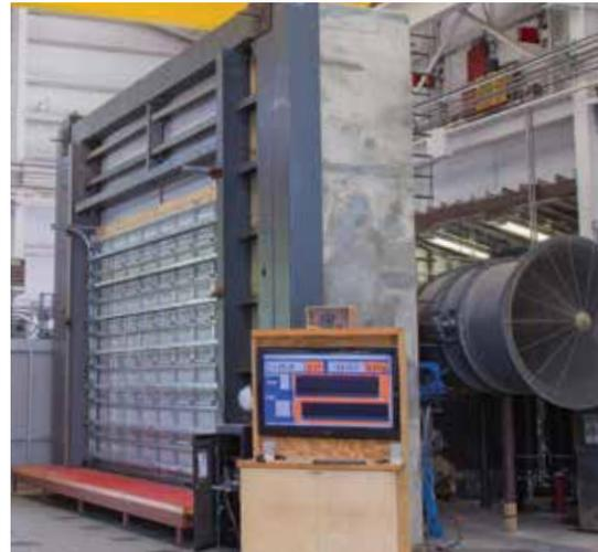
Sectional roll-up door installed prior to test.
