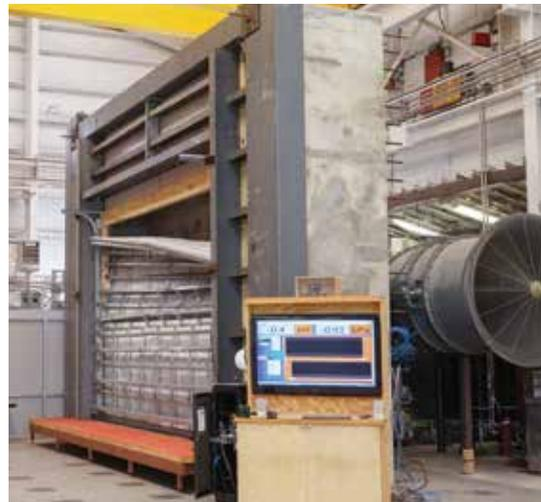
Damaged sectional roll-up door after test.
