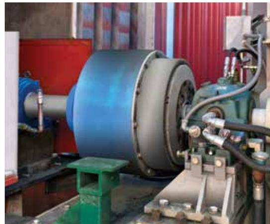
Wichita Clutch installed with drive ring.
