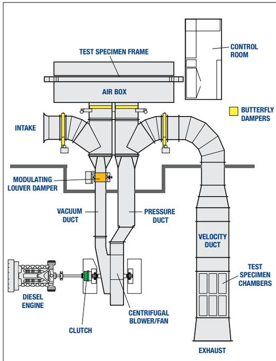
The Dynamic Wind Velocity and Pressure Simulator (DWVPS) is a unique machine that creates simulated Siffar-Simpson Scale Category 5 pressure events.
