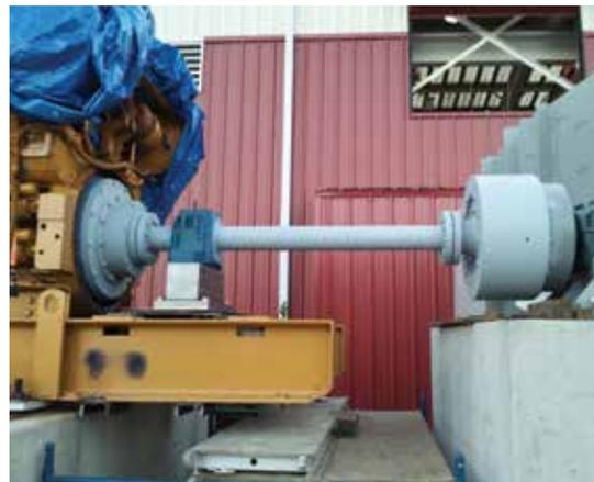
Engine/Blower drivetrain features (left to right), engine, coupling, bearing assembly, shaft drive ring, Wichita clutch, bearing assembly and blower assembly.
