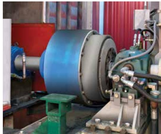
Wichita Clutch installed with drive ring.
