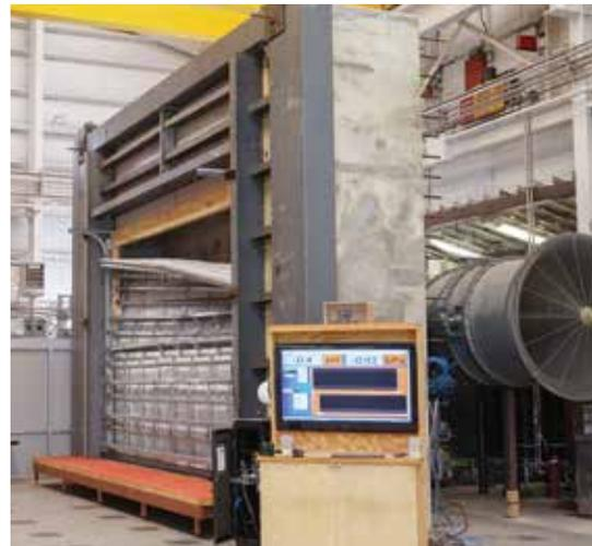
Damaged sectional roll-up door after test.
