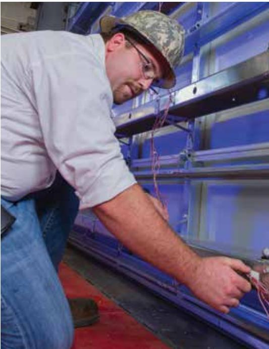
Strain gauges are attached to subject door prior to testing.
