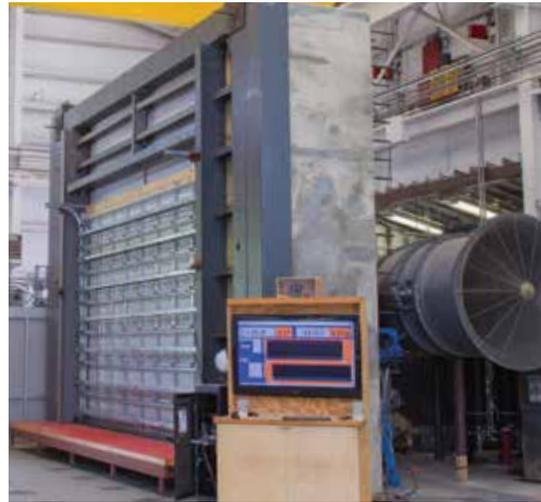
Sectional roll-up door installed prior to test.
