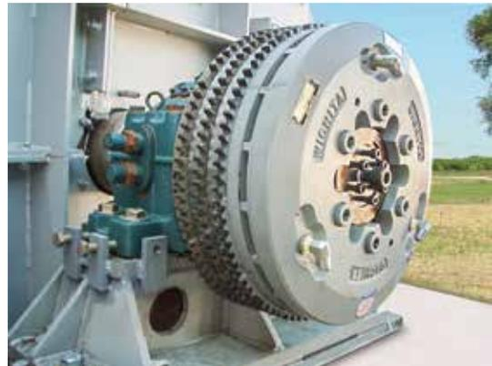
Wichita ATD-321-X Standard Ventilated Clutch mounted to bearing assembly adjacent to blower.
