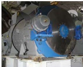
Twiflex Model GMR-SD caliper brakes shown operating on a drag motor disc.
