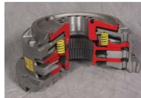
Heavy-duty LKB brakes feature high-energy metallic linings with large swept areas to ensure excellent heat dissipation, uniform stopping distances and long lining life. Units also feature high-strength alloy steel drive studs, actuation springs sized for maximum life, and long-life piston seals. Long spline lengths on the brake discs maximize load-carrying capacity.
