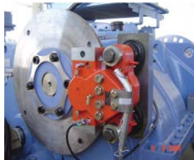
A Swendborg Model BSAK 3000 caliper brake is shown mounted to a wind turbine rotor disc.
