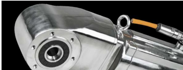
The IE4 super premium efficiency stainless steel geared motor is designed with surfaces which slope by at least 3° to prevent the formation of dirt deposits and allow the run-off of cleaning agents and water. Stainless steel construction eliminates the risk of the hygiene rating becoming compromised in the event of an impact or over prolonged periods of use in heavy washdown environments.
