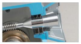
When a mounting position is selected where the input shaft is at or below the lubricant level, the configurator automatically selects dual input seals for added protection against leaks.
