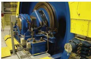
Twiflex Model VMS3-SPS caliper brakes installed on a 20 ft. diameter double-drum, single-clutch hoist at a Canadian gold mine.
