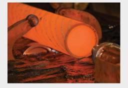
**Problem:** A leading Midwest seamless tube piercing steel mill was experiencing repetitive OEM universal joint knuckle failures on their mandrel and piercing mills. The original OEM universal joint knuckles would catastrophically fail without warning, turning rollers and other component fragments into projectiles which created a major safety concern. Failures were unpredictable, with some breaking down in days, weeks, or months, creating substantial delays and often shutting down production.
