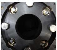
Standard on the MS series, the interlocking flange arrangement utilizes the fasteners in clearance holes to allow components to shift slightly in the event of a disc pack failure and act as a simple pin & bush coupling.
