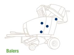
Tension control brakes from Warner Electric are used on netwrap drives.
