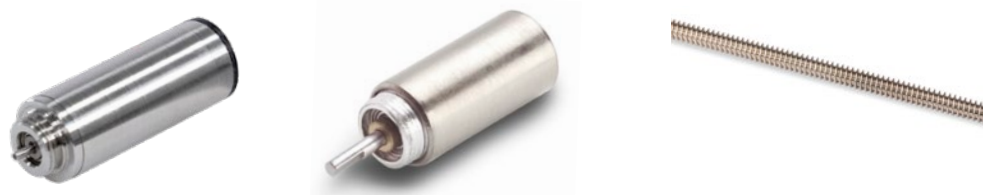
Figure 3: The 08ECP20 slotless BLDC motor, paired with the R08 gearhead and CM2150-1450N-A00A00-AFM lead screw deliver compact, high-torque linear motion ideal for fast, reliable tube decapping.
