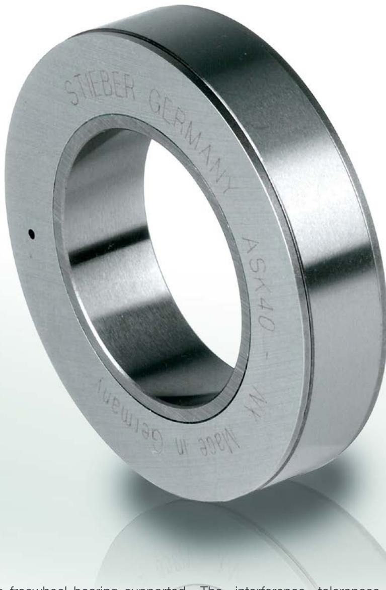
Type ASK is a roller type freewheel bearing supported by two rows of roller bearings. It is a self-contained dust protected unit, delivered grease lubricated.
