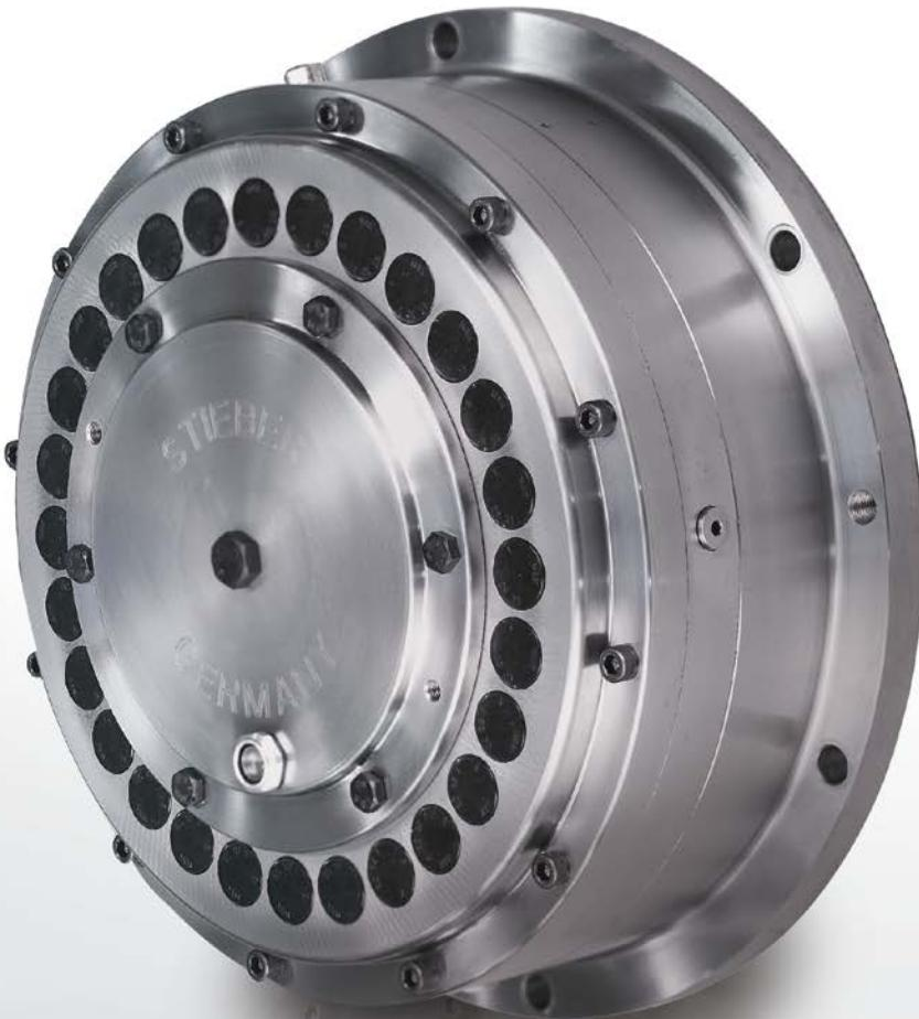
The type RDBK is a centrifugally lift-off sprag RSCI high speed backstop (Please refer to pages 72 to 75) equipped with integral torque limiter. The latter limits the backstop transmissible torque to a value that is factory set-up according to customer request.
