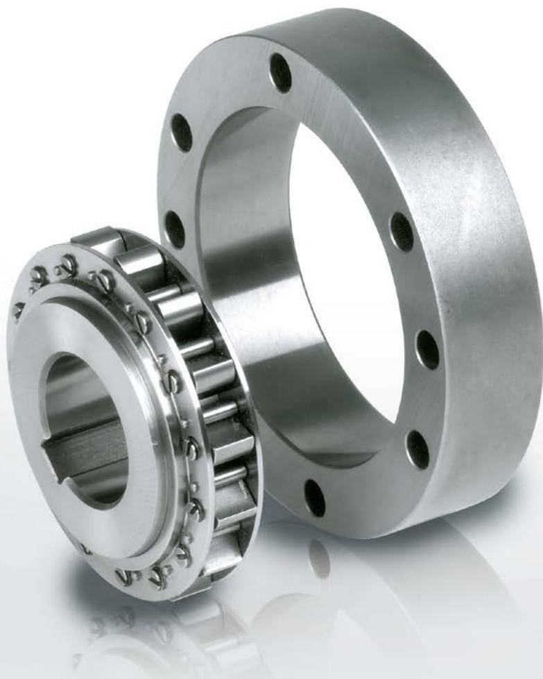
The series RSXM completes the small to medium backstop range, which commenced with the highly successful RSCI programme. Type RSXM is a centrifugal lift off sprag type freewheel with the inner race rotating. Only the inner race is designed for freewheeling. It is a non self-supported type. Bearings must be provided to ensure concentricity of the inner and outer races and support axial and radial loads, as shown overleaf. Concentricity and run-out limits must be observed.
