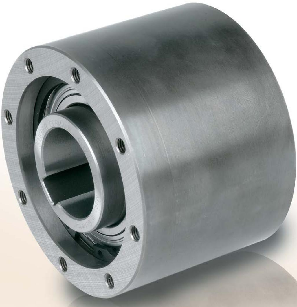
Type SMZ is a sealed, sprag type freewheel, bearing supported using two 60..ZZ series grease lubricated bearings.
