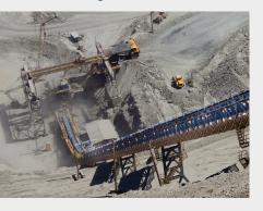
**Problem:** Most accidents on mining conveyors are caused by the stored energy in the belt. If not properly protected, a loss of power at a mine can allow loaded inclined conveyors to reverse direction, causing damage to expensive equipment. Reverse rotation of conveyor belts can be prevented by installing a standard backstop or a torque-limiting backstop. However, to allow the crew a safe maintenance routine, a loaded conveyor belt needs to be slowly rotated backwards to clear the belt.
