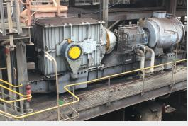
**Problem:** A major energy company in Australia needed reliable replacement low-speed backstops (LSBs) for use on six incline conveyors that move coal out of a mine to an adjacent power station. The existing LSBs were being removed every two years for inspection and often needed to be replaced due to premature failure.
