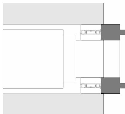
Pressing in or on by means of mounting aid (tube or bushing)
