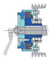
**Stromag KMK** as a shaft-pulley connection for use outside gearboxes (dry operation).
