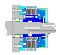
**Stromag KMK** for use in gearboxes (wet operation) with optional disc oil flushing.
