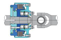
**Stromag KMK** as a shaft-cardan shaft connection for use outside gearboxes (dry operation).
