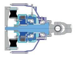
**Stromag KHR** as a "Two in One" combination in SAE housing on diesel engine with direct flange-mounted cardan shaft.
