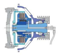
**Stromag KHA** with additional carrier for heavy-duty pilot bearing and bracing springs for reducing drag torque.
