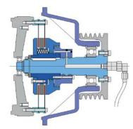
**Stromag KHM** for engine mounting. Backlash-free power transmission via diaphragm guided pistons and friction linings. Drag torque free when open.
