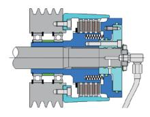
**Stromag KUK** as a shaft-pulley connection for use outside gearboxes (dry operation).
