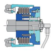
**Stromag KUK** as a basic type. For use outside gearboxes (dry operation).
