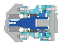
**Stromag KMB.ZM** mounted between gearbox and hydraulic motor.
