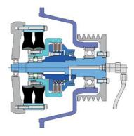
**Stromag KHA** with flexible Periflex®VN couplings for drives particularly subject to torsional vibrations. Connection for SAE flywheels.
