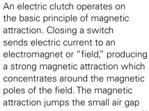
between the field and the rotor, effectively making the rotor a spinning magnet. This "magnet" attracts the armature, grips it tightly and causes it to turn with the rotor. Opening the switch turns off the magnet, disengaging the clutch.
