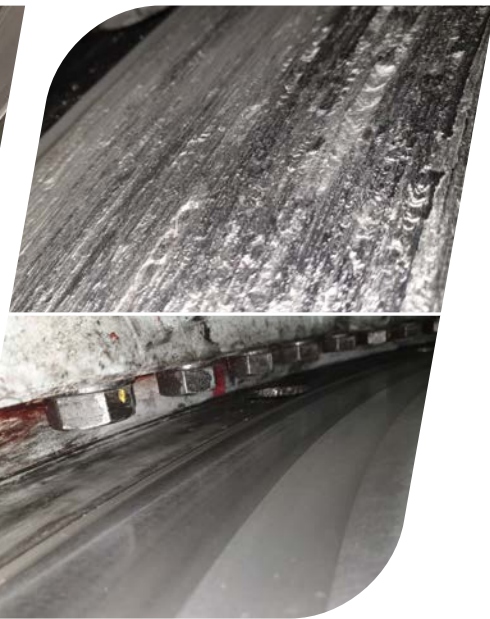
Top: Disc surface before milling. Bottom: Disc surface after DRT gen2 milling.
