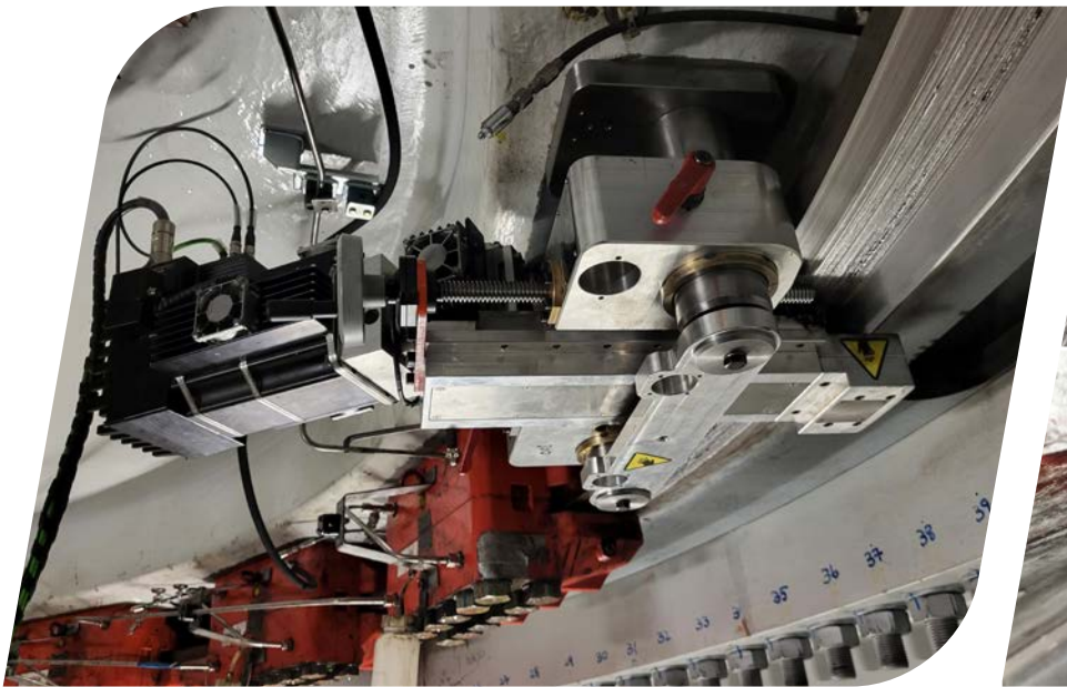
Svendborg Brakes DRT gen2 tool was mounted to mill the damaged disc surface.
